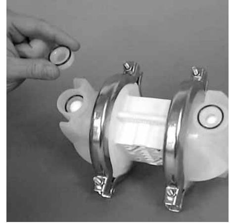
Step 6. Figure 6 Remove and inspect the seat, seat O-ring, and valve ball. Check for nicks, gouges, chemical attack or abrasive wear. Replace worn parts with genuine Wilden parts for reliable performance. (Figure 6)
