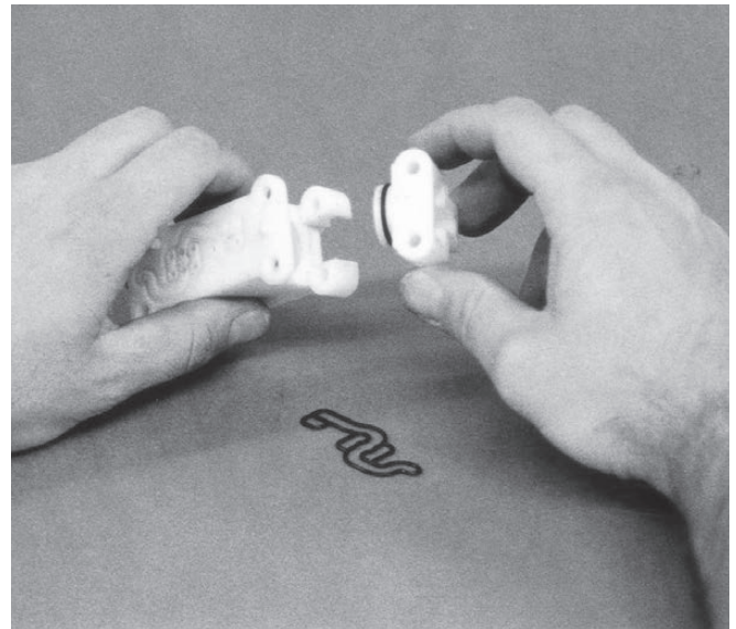
Step 3. Figure 3 Remove air valve end cap by simply pulling it away from air valve body (no tools required). ( Figure 3 ) Inspect O-ring and replace as needed with genuine Wilden parts.
