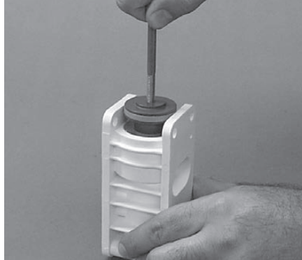
Step 5. Figure 5 Remove air valve spool from air valve body by threading one air valve bolt into the end of the spool and gently sliding the spool out of the air valve body. Inspect seals for signs of wear and replace entire assembly if necessary. Use caution when handling air valve spool to prevent damaging seals.
